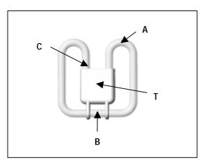
The maximum temperature on the plastic housing (T) should not exceed 90°C in order to maintain the rated lamp life. This requirement indirectly sets the operating environment, size and type of the fixture that the product operates within. For optimum performance in a fitting, consideration must be given to the heating effect of the lamp.
