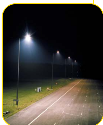
Night-time testing of the Starsense system to investigate the benefits of motorway lighting management.
