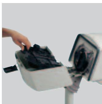
Removing the gear unit.
